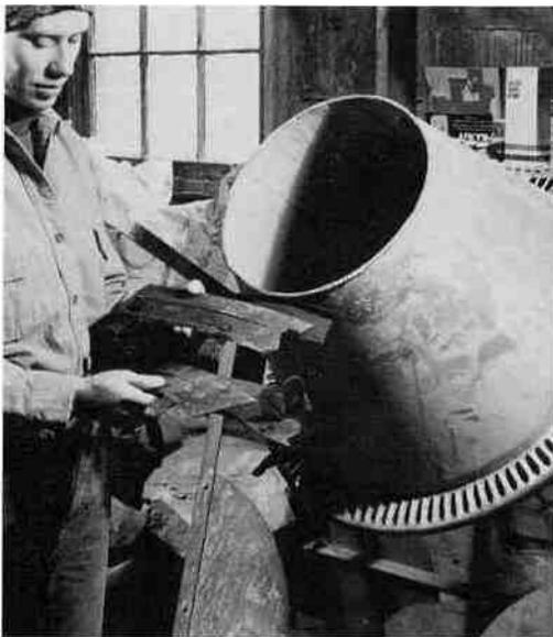
**Above** A backyard cement mixer can be altered to process clay satisfactorily. The four mortar-mixing blades are removed and the two top holes sealed with nuts, bolts and washers.
