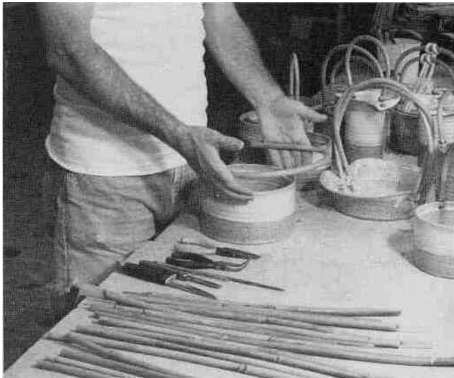
After soaking for two weeks, the wet cane is bent to an appropriate shape.
