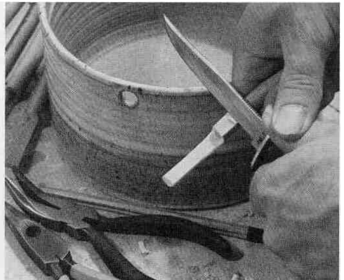
The doubled-back strap will nestle in an indentation carved above the routed cutout.
