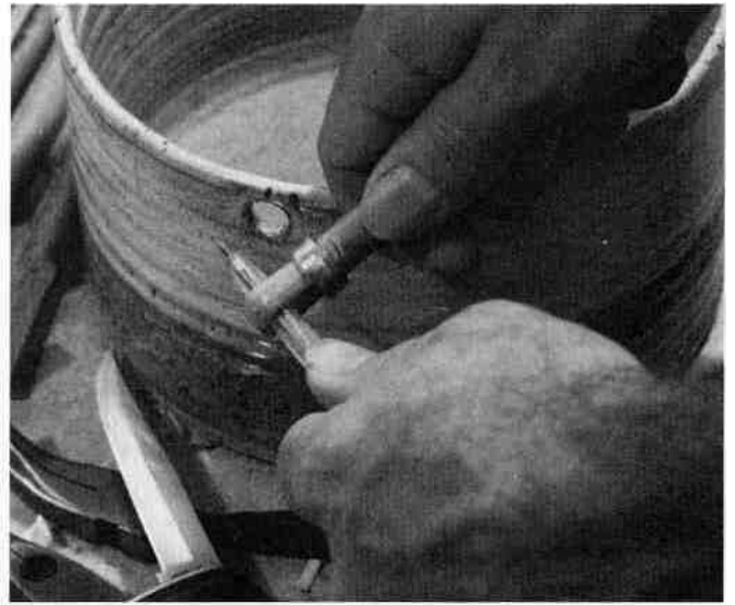
Folded over a ballpoint pen, the doubled-back strap is secured with a copper ring.
