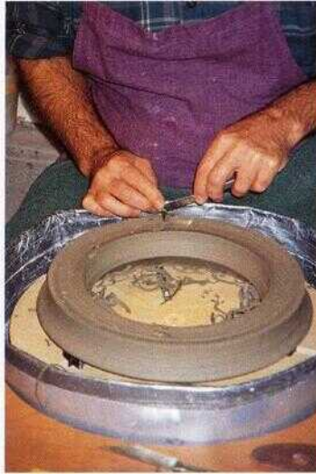
When the ring is leather hard, it is inverted and trimmed.
